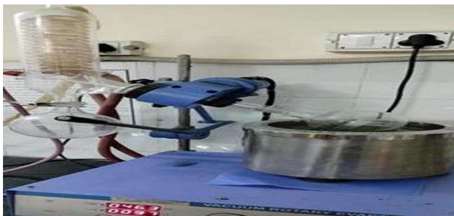
Figure 11: Rotary Vacuum Evaporation Process of P. niruri Ethanolic Extract.
